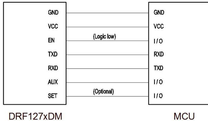
Figure 1: Pin Connections in Standard Mode
